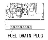
Unscrew the fuel drain plug. Reinstall the drain plug, after draining water completely
